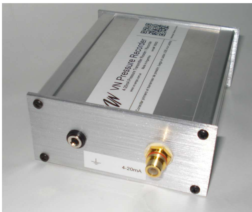
Unidad "Hardware" Pressure Recorder lado conector 4-20mA
